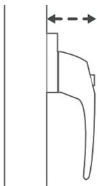
The 'Depth' of your chosen blind is simply the distance which the blind protrudes from where it's fitted. You'll need to know this depth to make the correct allowances when measuring:
