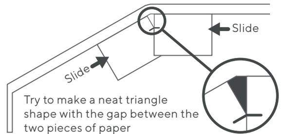
**3** Follow the edge of the paper back to the frame, and make a mark where each piece of paper meets the frame.
