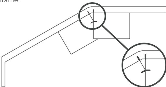
**4** The width from one mark to the next is the width you'll order each blind. For the left and right blinds, measure from the inside mark over to the wall (mark A in the below diagram). For the centre blind, measure mark to mark (B to B below).
