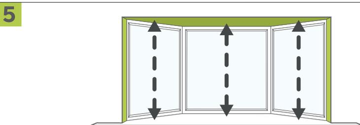
Measuring the drop is simple - simply measure from where the top of the blind is going to sit, down to where you'd like the bottom to rest (usually the sill, if there is one).
