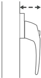
The 'Depth' of your chosen blind is simply the distance which the blind protrudes from where it's fitted. You'll need to know this depth to make the correct allowances when measuring. Regardless of which bracket you use, you'll need it to be at least 75mm away from the frame. Top fix brackets are all standard, while longer face-fix brackets are available by request:
