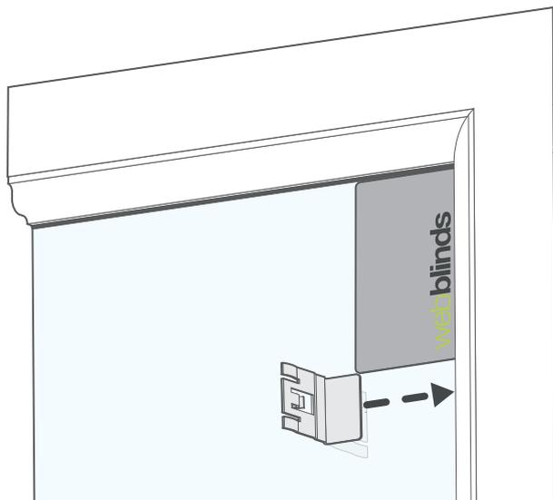
Locate the correct position for the brackets by holding a credit card or store card vertically in the corner of the glass - the bracket will sit in line with the edge of the card.
