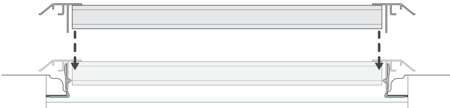
Push the frame towards the window until the oval slots lock onto the prongs of each of the brackets. The installation of the blind is now complete.
