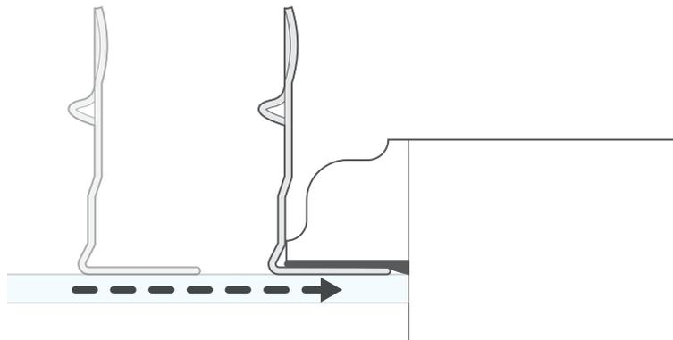
Push the bracket firmly into place between the glass and the rubber seal.
