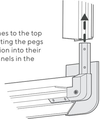
Tighten the two screws already inserted into the locating pegs on each corner piece. Repeat the process for each corner.
