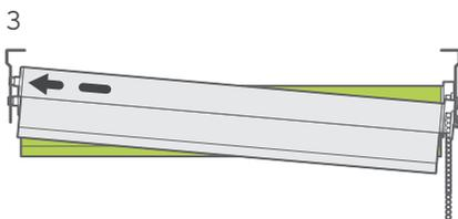
Repeat the process for the front blind placing the pin into the cross-shaped hole on the bracket and lifting the sidewinder side up to slot into the cross section.
