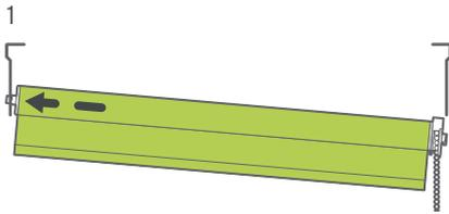
Install the rear blind first. Begin by placing the spring-loaded pin into the lower cross-shaped hole on the bracket. Push the blind toward the bracket so the spring-loaded pin depresses.
