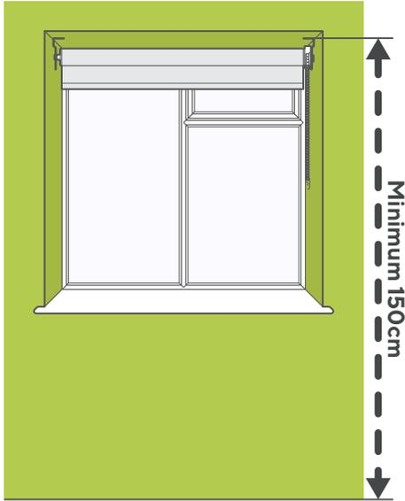
For safety reasons, always ensure that the top of the blind is installed at least 150cm (1500mm) from the floor.
