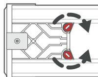
At the end of the rail opposite to the lever there is an adjustment block that allows you to fine-tune the fitting of the rail. Use a flat-head screwdriver to twist the small red plugs **in** toward the centre of the rail. Slide the block out of the rail by a few millimetres, then twist the red plugs back into their original position to fix the block in place. **Make small adjustments only**, repeating as necessary for a tight fit.
