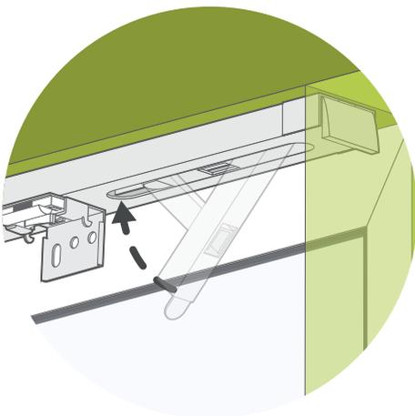
Hold the Click 2 Fit™ rail up against the top of the recess, then push the lever firmly upwards until the rail snaps into place. If the rail is not quite tight enough then this can be easily adjusted:
