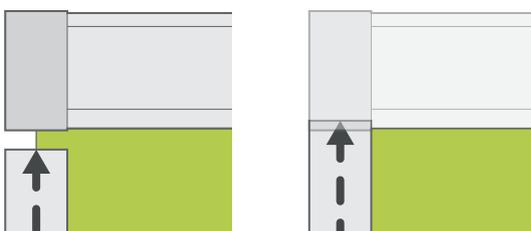
Slot the channel into place just under the cassette fascia (there is a small tab to guide the channel into place - the front of the channel should site between the fascia and this tab).
