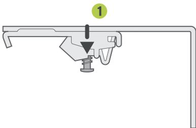
Loosen the screw in the centre of the top of the bracket enough to allow the locking part to move back and forth.
