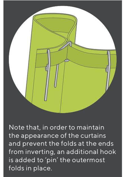
Note that, in order to maintain the appearance of the curtains and prevent the folds at the ends from inverting, an additional hook is added to 'pin' the outermost folds in place.
