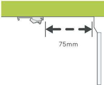
If you are using top-fix brackets, the front edge of the bracket must be at least 75mm (3") away from the facing surface behind the rail. This will ensure that the waves in the fabric do not brush against the wall or window behind.
