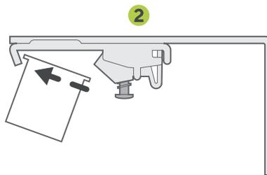
Locate the front lip of the curtain headrail into the front hook of the bracket.
