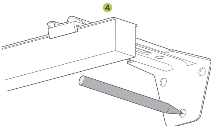
Place the rail and brackets up against the fixing surface and mark out the screw locations with a pencil.
