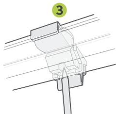
3 Hold the rail up to the fitting surface and mark out the screw holes with a pencil.
