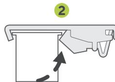
2 Rotate the headrail so that the back lip slots into the locking part of the bracket.
