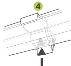
4 Put the rail safely to one side and drill holes where you marked out the brackets, then insert a rawl plug into each hole. Use a single screw for each bracket, through the centre hole in the top of the bracket.
