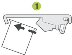
1 Locate the front lip of the curtain headrail into the front hook of the bracket.
