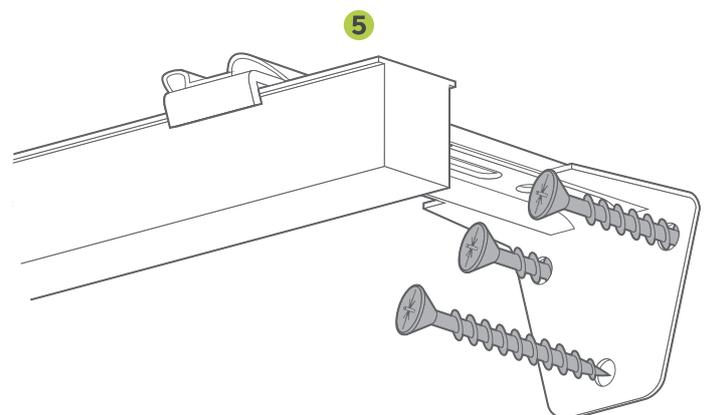
Put the rail safely to one side and drill holes where you marked out the brackets, then insert a rawl plug into each hole. Use a single screw for each bracket, through the centre hole in the top of the bracket.
