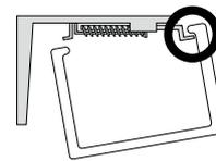
1. Locate the front lip of the rail onto the front lip of the brackets, hold the rail at a slight angle while doing so.
