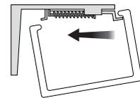
2. Push the rail towards the back of the bracket whilst still holding it at a slight angle. The springs will contract and only a small amount of pressure is required.
